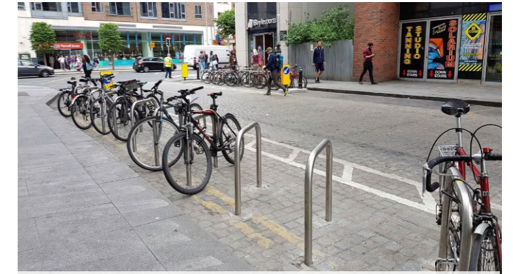
Cycle stand parking set back from the pedestrian thoroughfare with different paving, against a surface colour and texture change.
