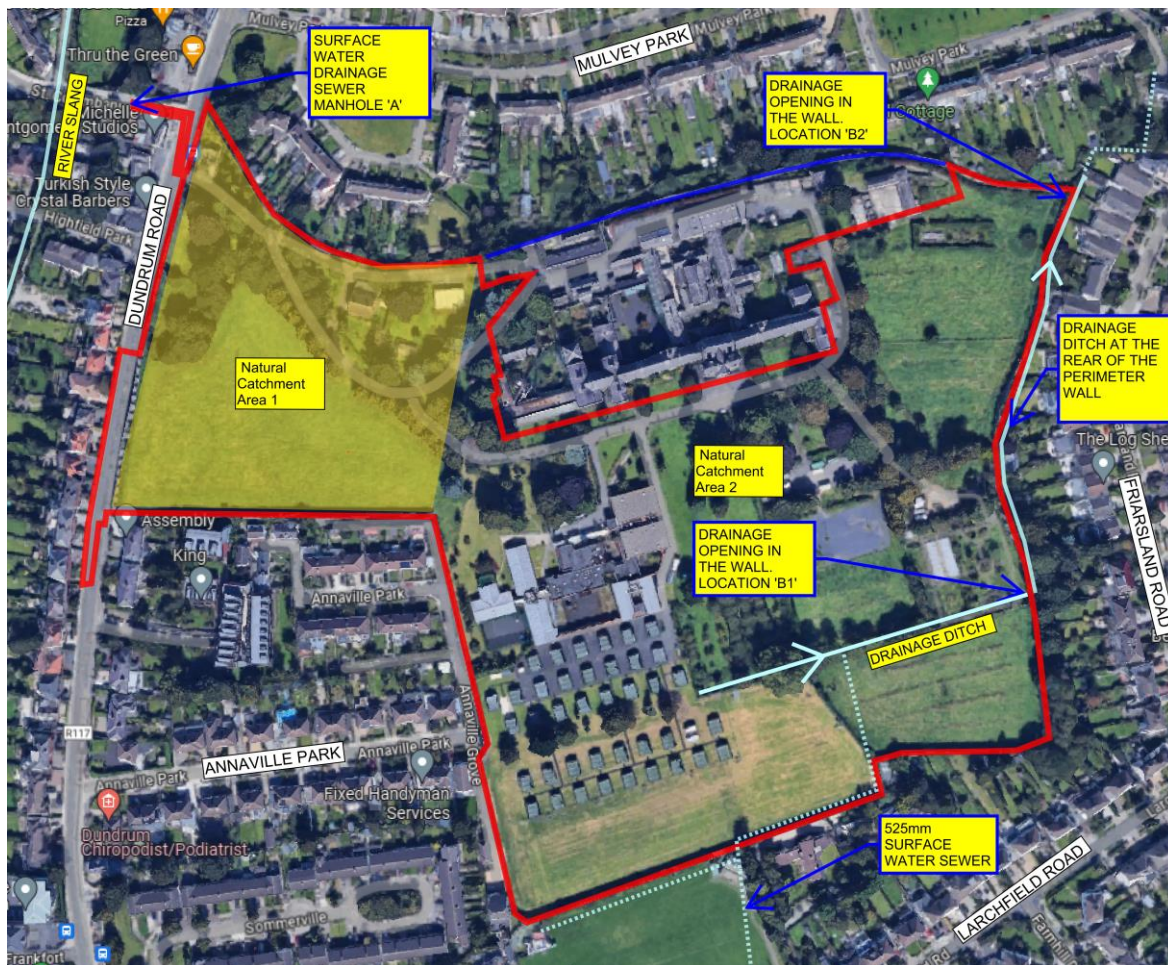
Fig 3.1. Aerial View of the Approximate Natural Catchment Areas and surface water drainage outfalls on the Existing Site. Catchment 1 shaded yellow. Catchment 2 is in the unshaded area.
